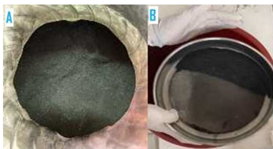
Fig. 1 The crushed shells before (A) & after (B) sifted using a 100 mesh sieve.
