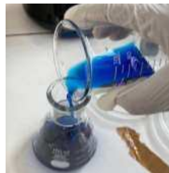
Fig. 2 Mixing the adsorbent with a 20 ppm methylene blue solution.
